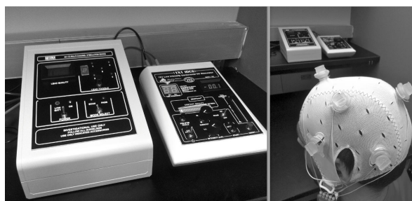
Figure1: 4x1-Ring High-Definition Transcranial Direct Current Stimulation (HD-tDCS). Left: Multichannel Stimulation Adaptor (L) connected to 1x1 Low-intensity DC Stimulator (R). Right: Electrode positioning.
